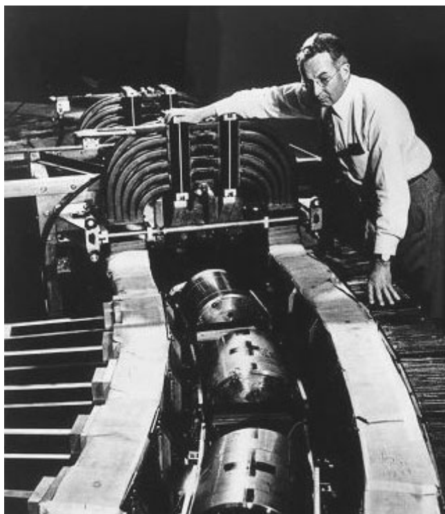
Fig. 5. While chairman of the division of physics, mathematics, and astronomy, the physicist Robert F. Bacher initiated construction and use of a new electron accelerator, called a synchrotron, shown here. In 1962, he became Caltech's first provost. Caltech Archives.
