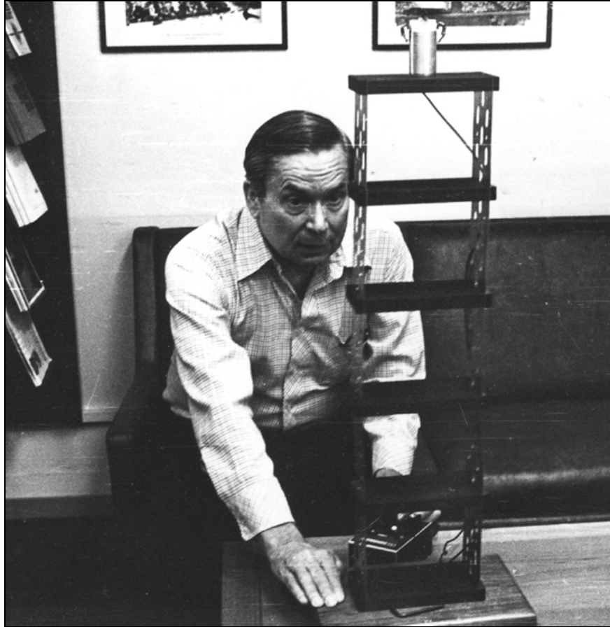
George W. Housner controls the frequency of a rotating shaker atop a simple five-story building model (1978).
