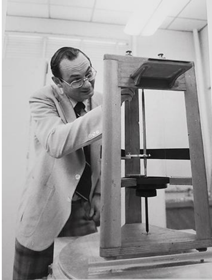
Jennings in 1979 makes an adjustment to a seismometer, an instrument that registers the ground motion associated with earthquakes. Caltech Archives Photo
