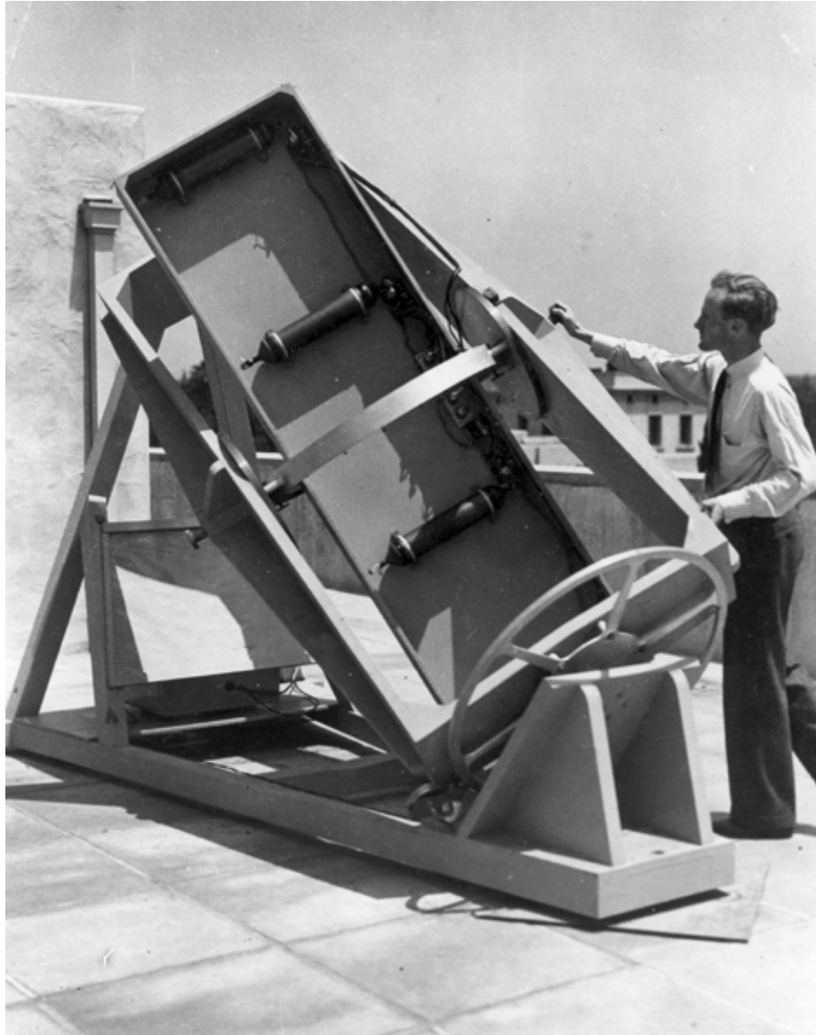
Fig. 1. William Pickering uses an experimental telescope to investigate the source and intensity of cosmic rays on the roof of Robinson Laboratory of Astrophysics, ca 1939-1942. Electrical circuitry linking three cylindrical ion chambers, mounted parallel to the telescope's axis, allows the simultaneous detection and measurement of high-energy cosmic ray particles. Caltech Archives.
